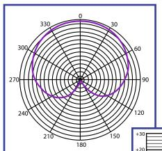
Designed exclusively for iCOM radios, the iC Electret element has a -3dB fixed point at 35 Hz and 12kHz with the sensitivity of-48 at 1500 ohms output centered at 1kHz. The iC element solves the problems with LOW GAIN ICOM radios but can also work with great results on newer Icom models. Bias power is applied to operate the iC electret element. The Pro 7 iC is supplied with our ADI-IC eight pin Icom adapter cable.
